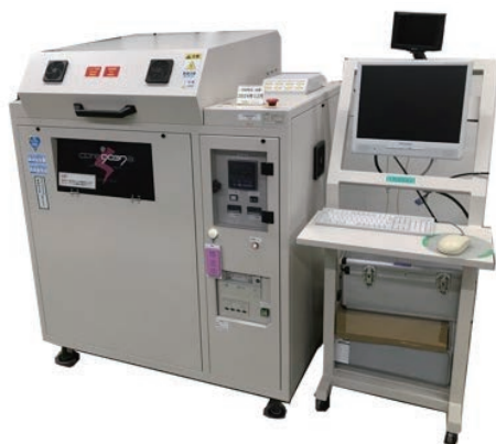
Warpage evaluation during reflow of module products
