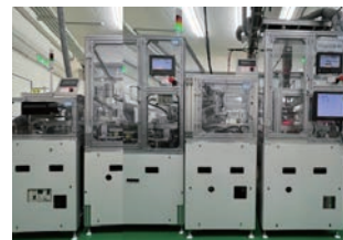
Testing-resin coating-curing integrated production line
