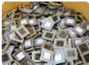
Disassembled and Separated ICs
