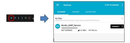
(6) Tap the "CONNECT" button in the application to connect via Bluetooth®, then tap the "DISCONNECT" button to disconnect. You will see that it stops at the breakpoint (disconnect process) set in the previous section of the source code.
