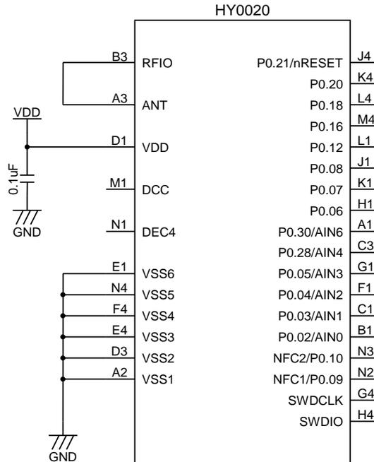
Figure 5-1 Built-in LDO regulator circuit example
