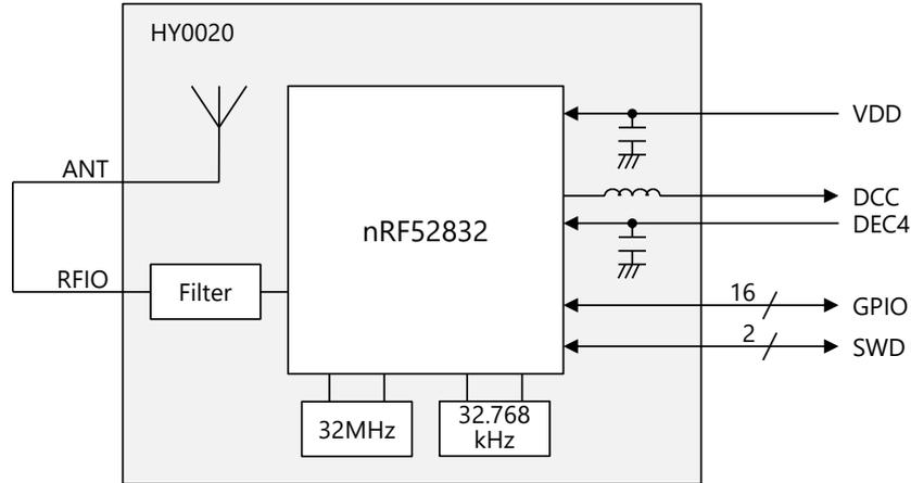
**Figure 3-1 Block Diagram**
