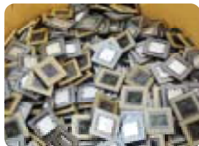
Disassembled and Separated ICs
