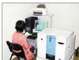
Analysis of chemical substances using an X-ray fluorescent spectrometer
