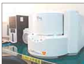
An X-ray fluorescent spectrometer
