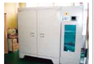
Measurement of VOCs emitted from large-sized equipment (home electric appliances and PCs)
