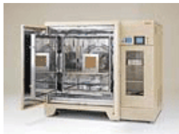
VOC emission measurement chamber (1,000 L) (VOC-10) Made by Espec Corporation
